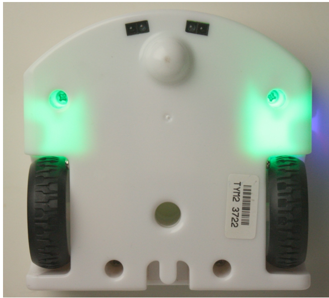
Figure 3.1: The bottom of the Thymio with two ground sensors at the front
